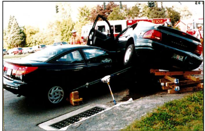
Vehicle Stabilization at an accident.
